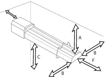
Note: Dimension "C" indicates the minimum required safe distances from combustibles, it DOES NOT indicate the required mounting height. The minimum mounting height is 7 feet, except for aircraft hangars and public garages.
