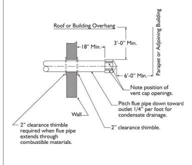
Double Wall Double wall vent run and Double wall terminal end
