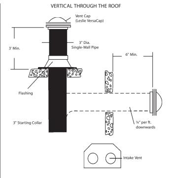
The air supply duct may have to be insulated to prevent condensation on the outer surface. The outside air terminal should be securely fastened to the outside wall by drilling four (4) holes in the outside flange; wood screws or bolts and expansion sleeves may be used to fasten terminal.
