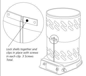
STEP 4: LOCK THE CLIP INTO PLACE WITH 3 SCREWS AS SHOWN. THE HEATER MUST NOT BE OPERATED UNLESS THE OUTER SHELL IS PROPERLY EXTENDED AND FULLY LOCKED INTO PLACE.
