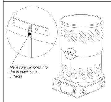
STEP 3: LIFT OUTER SHELL UNTIL ALL THREE CLIPS INGAGE SLOTS IN LOWER SHELL. WHEN THIS HAPPENS, THE SCREW HOLES WILL LINE UP.
