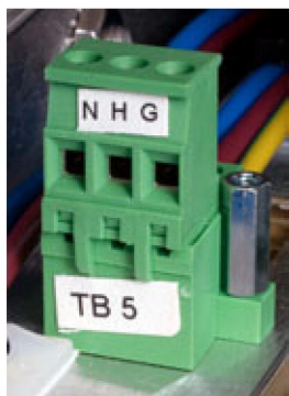
Figure 3-7: AC/DC termination block
