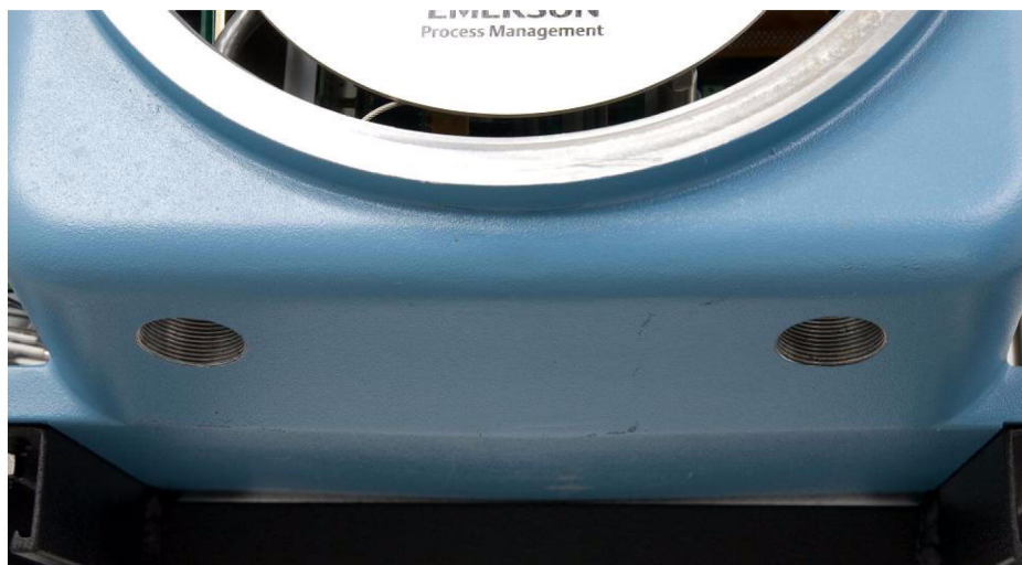
Figure 3-6: Location of entries for wiring on the under side of the lower enclosure
