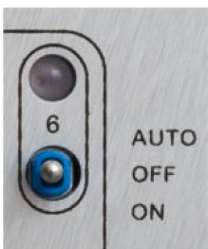
Figure 2-3: Valve switch from switch panel set to “OFF”
