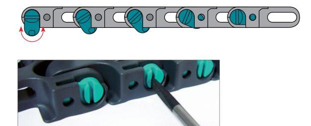
With a simple (but sufficiently large) flat screw driver, the clip can be twisted and taken out. Then the pin can be pulled out.
