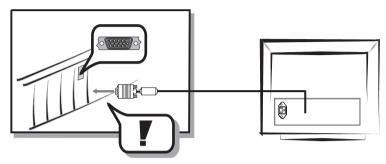
For connecting your monitor to a Macintosh computer, make use of the special adapter available from your dealer. See the chapter ('Connecting the monitor to a Macintosh computer') for information on the connection of this adapter and the dip switch settings.
