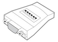
The optional adapter is for connecting your ELSA monitor to Macintosh computers. Set the DIP switches according to the table below.
