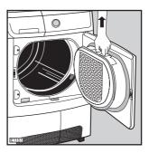
Do not be alarmed by the amount of fluff. It is not due to excessive wear caused by the dryer. All fabric loses fluff when drying but it goes unnoticed in the air. In a tumble dryer it simply collects in the filter.
