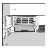
To pull out the condenser, first turn the two red stops downwards and then remove the condenser unit holding it at the handle.
