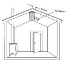
To mount onto a wall or ceiling, simple remove the battery compartment and mark the position of the two mounting holes. Drill two holes using a 6mm drill for the plastic plugs (supplied) and screw the unit home with the screws supplied
