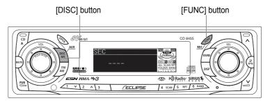
Press the [FUNC] button for more than one second. If the security code matches the code recorded by the deck, [OK] will appear on the display and the security function will be canceled.
