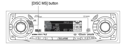
First press the [DISC MS] button for less than one second to switch to the disc mode. It is assumed here that a CD has already been loaded into the unit.
