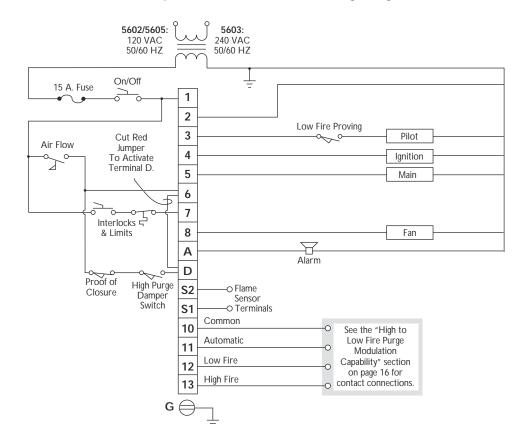
Figure 5.3 Typical Connections For All Models
