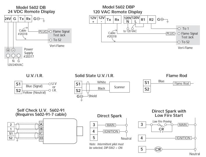
Note: Intermittent pilot must be selected, DIP-SW2 = ON CR is a control relay used to bypass the low fire switch after the burner is lit.
