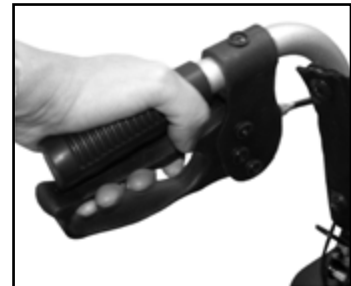
attendant wheel lock, temporarily locked
