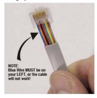
3. Insert the connector into the crimper, and crimp. Be careful no to push the connector too far into the crimper as the low profile connectors do not have a stop to position the connector at the correct position. Also be sure the wires are all of the way into the connector when you make the crimp. It is a good idea to crimp the connector twice to be sure that all of the conductor pins have pierced the wires.
