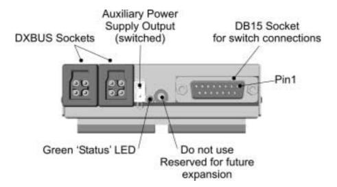
The DX-ARC-SWB connections are located along the front panel of the case. When all wiring has been completed, it must be securely fastened to the powerchair frame to ensure there is no strain on the connectors.
