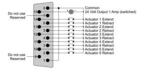
'Normally-open' switches should be used so the required function operates on switch closure between the appropriate pin and **Common** (pin 8 of the connector).
