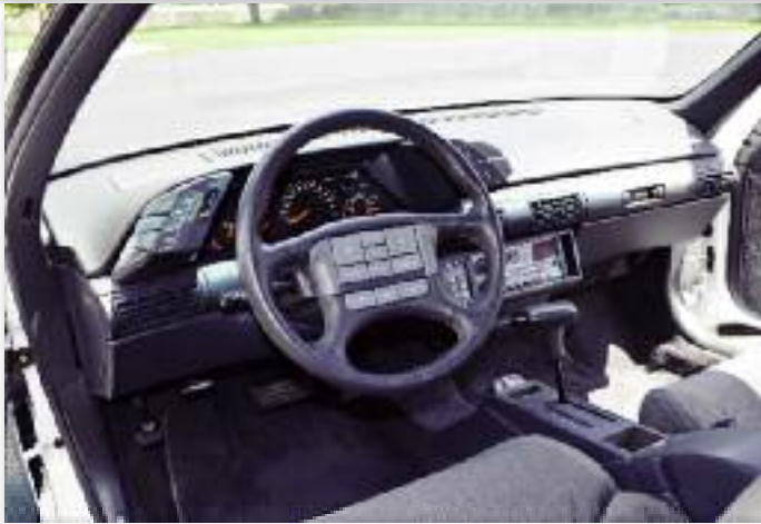
The dash design of the '92 GP featured full instrumentation in lieu of the usual "idiot lights." This design also featured stereo controls in the steering wheel. Note the combination lock on the glovebox door.
