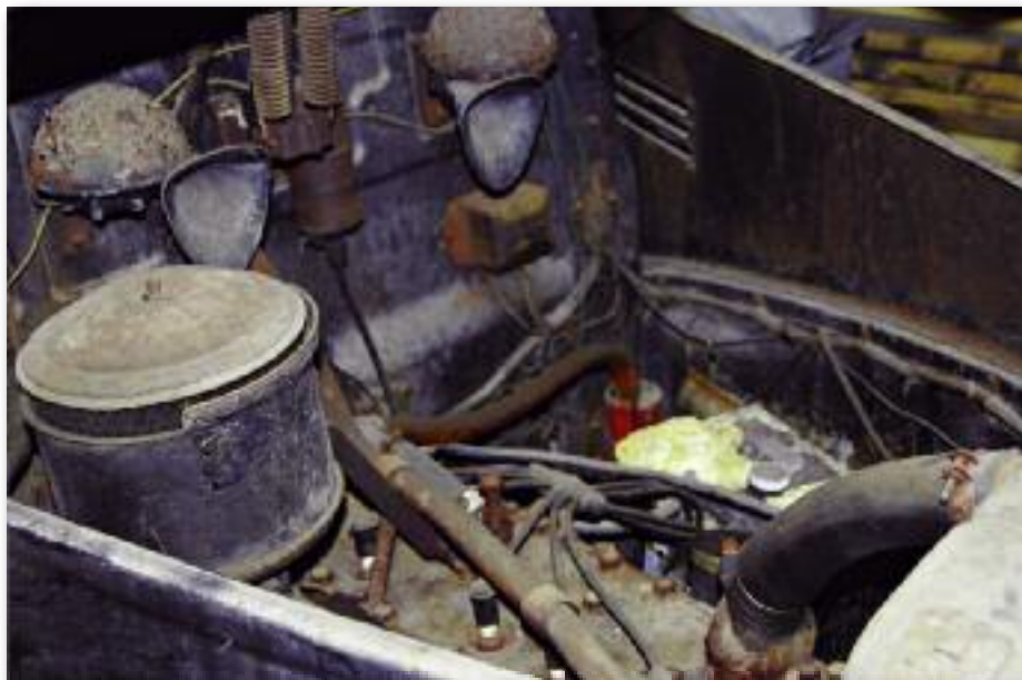
Check out the acid build up on the battery.
