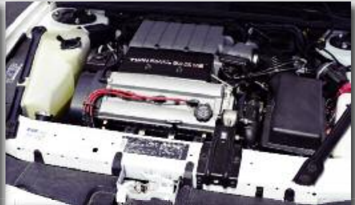
This Twin Dual Cam V-6 was the standard motor in the special edition cars. Features include electronic multi-port fuel injection, four valves per cylinder, four overhead cams, aluminum heads, heavy duty crank and high flow injectors. This combination produces 210 horsepower with the 5-speed manual transmission and 200 with the automatic.
