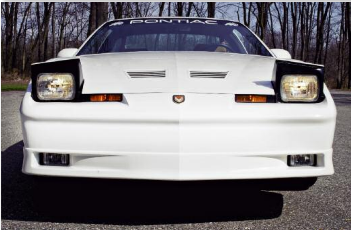
Though the nose of the '89 Turbo Trans Am looks like it would increase wind resistance with its relatively flat bumper face, it is actually much more slippery than one might think. Extensive wind tunnel testing made this design one of the most aerodynamic designs ever to come out of Detroit.
