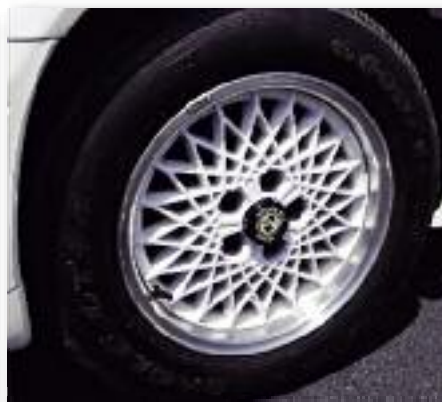
Special Richard Petty center caps are one of the features unique to the special edition. This car retains its original Goodyear GT + 4 tires on the cross-lace color coded wheels, also standard on the Richard Petty cars.
