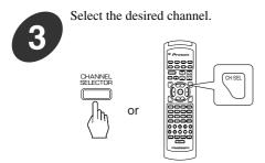
Each time this button is pressed, the corresponding channel is selected and displayed for 3 seconds as follows:
