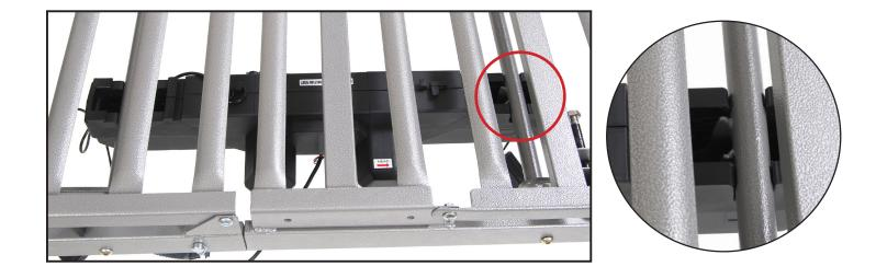
B6. Once in place, replace the motor covers to secure the motor.
