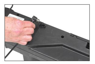
7. To install motor, remove locking caps on top of the motor.
