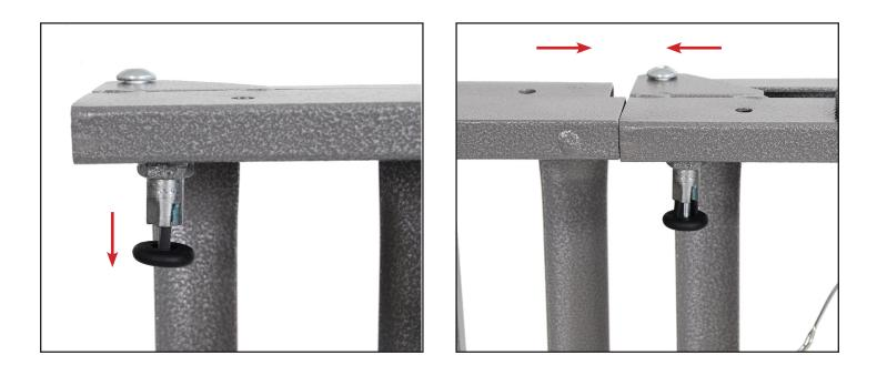
To disassemble the head and foot section, pull the black lock knob out and rotate the knob a quarter turn. The lock knob will remain open to allow the head section to be removed from the foot section.
