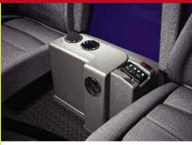
Compressor/evaporator/blower unit with molded composite cover fits between seats, discharges cool air toward driver, connected by flexible refrigerant linesets to condenser unit on back of cab or under truck. Digital control mounts on top of unit for easy driver access.
