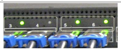
**Note:** Ports 3 and 4 illustrate a x8 connection with a single LED lit while Ports 5 and 6 illustrate two independent x4 connections with a LED lit for each port.
