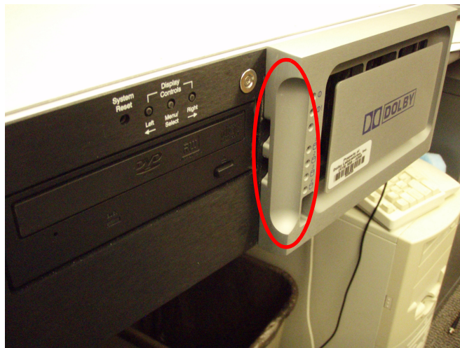
Figure 3-3 Locate Pry Areas Behind Drive Cover
