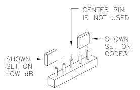
(Use needle nose pliers to pull and properly set the jumper plugs.)
