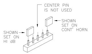
No jumper plugs are needed for Continuous Horn and low dB settings. However, it is recommended that the jumper plug be retained in the unit for future use (if needed) as shown in Figure 3, 4 and 5.
