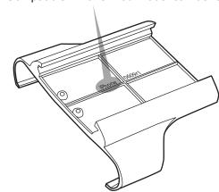
Each holder is designed for a different iPhone/iPod model. Identify the holder by the printed text on the back of the holder and choose the correct holder for your iPhone/iPod.
