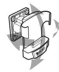
To adjust the angle of the cradle, please loosen the set screw enough for the cradle to move freely. When you are done adjusting the angle, hold the base and tighten the set screw. DO NOT OVER TIGHTEN!
