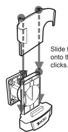
Slide the correct holder onto the cradle until it
