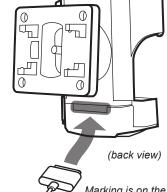
Attach the iPod dock cable into the connector on the back of the cradle
