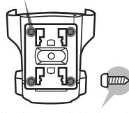
Use the screws (x4) in the package to screw the cradle to AMPS standard mounts.
