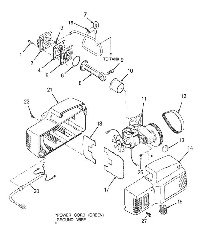
Slide #19 over #7 as shown. Make sure that no part of #7 tube touches #21 or #14 shroud when assembled.
