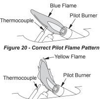
Figure 21 - Incorrect Pilot Flame Pattern
