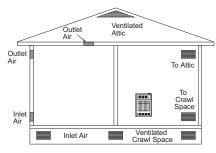
Figure 3 - Ventilation Air from Outdoors
