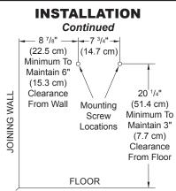
Figure 5 - Mounting Screw Locations
