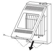
Figure 10 - Removing Front Panel Of Heater
