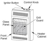
Figure 1 - Vent-Free Gas Heater
