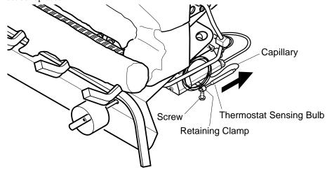
Figure 28 - Removing Thermostat Sensing Bulb
