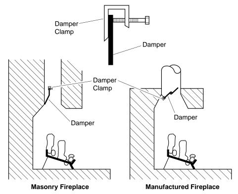
Figure 10 - Attaching Damper Clamp
