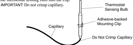
Figure 32 - Positioning the Thermostat Sensing Bulb in the Vertical Position with the Capillary at the Bottom
