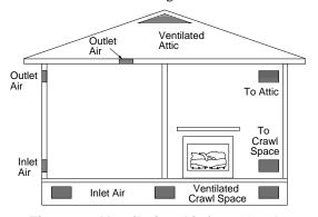
Figure 3 - Ventilation Air from Outdoors
