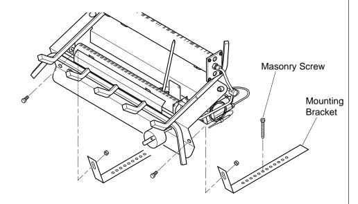
Figure 12 - Attaching Mounting Brackets to Heater
