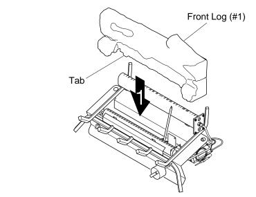
Figure 17 - Installing Front Log
