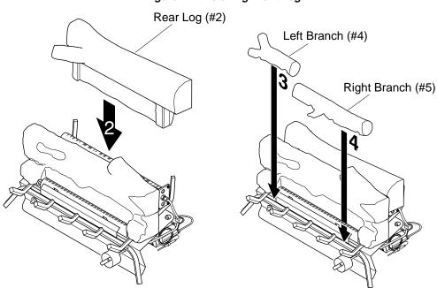
Figure 18 - Installing Rear Log
