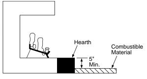
Figure 9 - Minimum Fireplace Clearances Above Combustible Flooring
