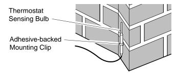
Figure 29 - Locating Thermostat Sensing Bulb on Masonry Fireplace
