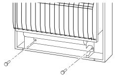
Figure 12 - Installing Bottom Mounting Screws
