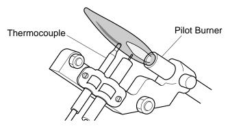
Figure 18 - Correct Pilot Flame Pattern
