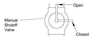
Figure 14 - Manual Shutoff Valve
