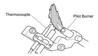
Figure 19 - Incorrect Pilot Flame Pattern
