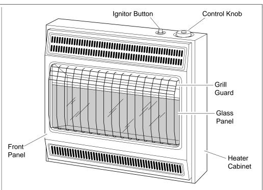
Figure 1 - Vent-Free Natural Gas Heater (28,000 Btu/Hr Model Shown)
