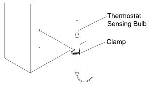
Figure 5 - Attaching Thermostat Sensing Bulb
