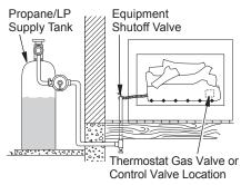
Figure 17 - Checking Gas Joints (Propane/LP Gas Models)
