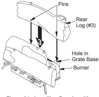
Figure 21 - Installing Rear Log #3 (CCL3930PTB/NTB Shown)
