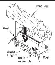
Figure 28 - Installing Front Log
