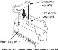
Figure 23 - Installing Crossover Log #5 (CCL3930PTB/NTB Shown)
