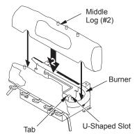
Figure 20 - Installing Middle Log #2 (CCL3930PTB/NTB Shown)
