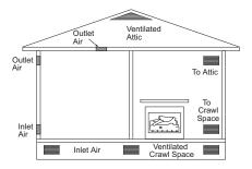
Figure 3 - Ventilation Air from Outdoors
