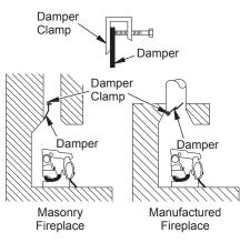
Figure 10 - Attaching Damper Clamp
