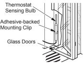
Figure 43 - Installing Thermostat Sensing Bulb Behind Glass Doors
