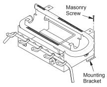
Figure 12 - Attaching Base Assembly to Fireplace Floor - Dual Burner Model
