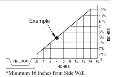
Figure 4 - Minimum Clearance for Combustible to Wall
