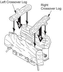
Figure 29 - Installing Left and Right Crossover Logs
