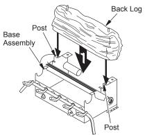
Figure 27 - Installing Back Log
