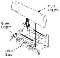
Figure 19 - Installing Front Log #1 (CCL3930PTB/NTB Shown)
