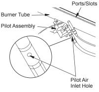
Figure 37 - Pilot Inlet Air Hole
