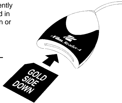
Figure 3: Inserting a SmartMedia Card
