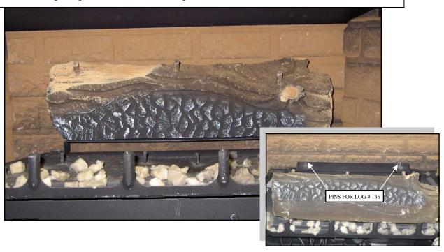
**STEP 3** - Locate log #137 and place onto the left side of the burner using locator pins and pre-drilled holes in log. Log will sit as shown in photo below.
