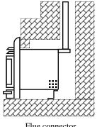
Flue connector straight-up vent
