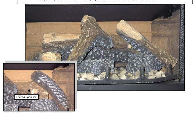
**STEP 8** - Locate log #138 and place onto rear log using the locator pins and pre-drilled holes in log. Log should sit behind left grate tine as shown in photo below.
