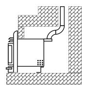
Flue connector offset vent
