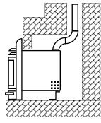
Flue connector offset vent
