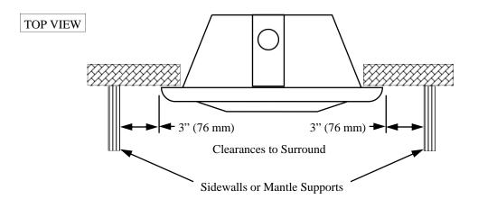
**CAUTION:** This appliance is designed for use in any masonry, factory-built wood burning and specific zero-clearance vented gas fireplaces (Due to constant additions, contact Archgard Industries for an updated list of suitable gas fireplaces). This appliance cannot be enclosed with combustible material and used as a built-in gas fireplace.
