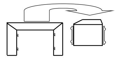
The surround has four hooks that clip onto the sides of the appliance. Make sure the surround sits evenly with the front of the fireplace. After the surround is properly installed, the bottom edge of the centre section of the surround is about 3/4" from the top of the appliance.
