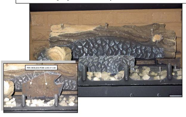
**STEP 5** - Locate log #141 and place onto right side of burner using the locator pins and pre-drilled holes in log. Log should sit as shown in photo below.
