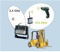
Fork-lift truck terminals with Datalogic RF readers
