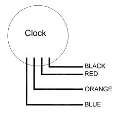
Connect to a good ground point in the vehicle Connect to switched 12 volt power point (An accessory terminal will work for this) Connect to a constant 12 volt power point (This will keep the correct time) Connect to the taillight circuit
