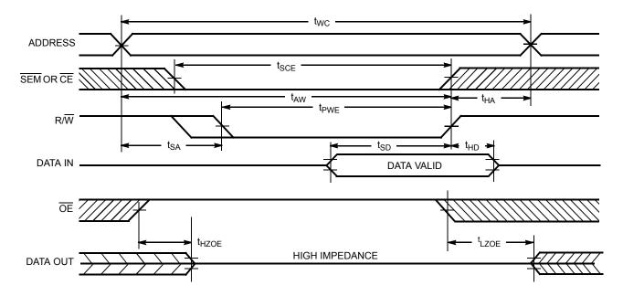
Figure 7. Write Cycle No. 2: R/W Three-States Data I/Os (Either Port)<sup>[22, 24, 25]</sup>
