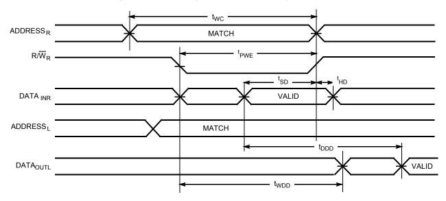
**Notes** 16. R/W is HIGH for read cycle. 17. Device is continuously selected  $\overline{CE} = LOW$  and  $\overline{OE} = LOW$ . This waveform cannot be used for semaphore reads. 18. Address valid prior to or coincident with  $\overline{CE}$  transition LOW. 19.  $\overline{CE}_L = L$ , SEM = H when accessing RAM.  $\overline{CE} = H$ , SEM = L when accessing semaphores.
