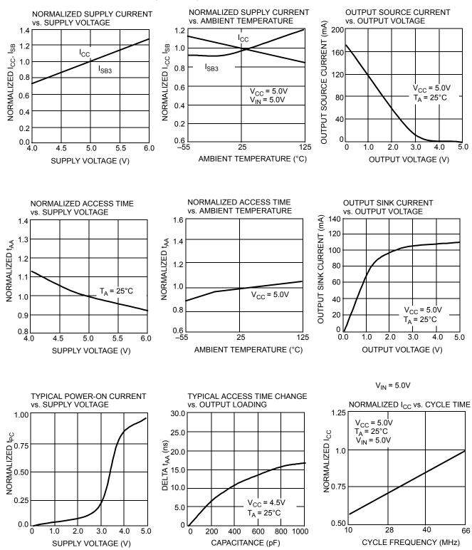
Figure 15. Typical DC and AC Characteristics
