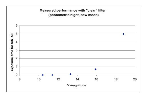
Figure 6. Exposure time calculator for the CCDS acquisition camera with the "clear" filter. Performance measured on a clear night with no moon. Note that objects are detectable with a  $S/N\sim10$ : the above exposure times are an overestimate of the exposure time for minimum detection.
