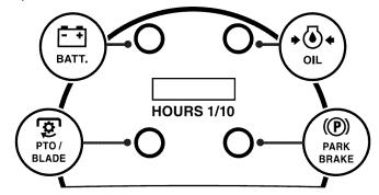
When the ignition key is rotated out of the STOP position but not into the START position, the system's indicator monitor displays the battery's output, in volts, on its LCD for approximately five seconds, after which it displays an hour glass and the hours of tractor operation. Once the tractor is started, the monitor continually displays an hour glass and the hours of tractor operation on its LCD.
