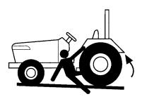
Do not allow anyone but the operator to ride on the tractor unless a passenger seat is fitted. Keep bystanders away from the tractor during operation.
