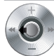
Exiting after selecting ROC EQ Move the lever towards << or press the Play button. Adjust 5Band dB levels Either press short on the lever or push it towards >> to adjust 5Band dB levels.
