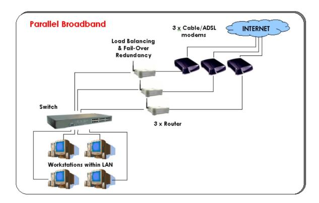
To implement Parallel Broadband, you will need to install two or more units of the router in the network, each connected to its broadband Internet service account. There is no restriction to the type of broadband Internet accounts they are connected to (whether Cable or ADSL). You may thus have one router connected to Cable Internet, and another to an ADSL line.
