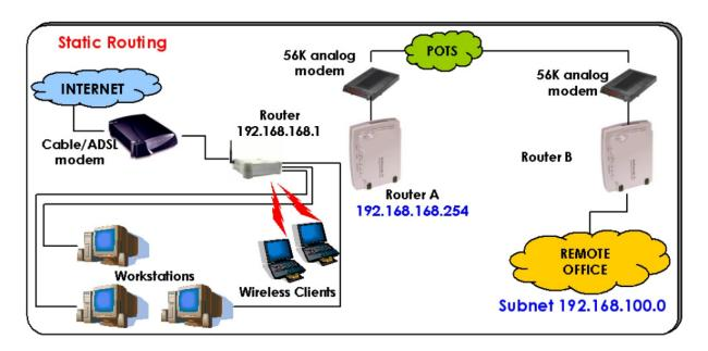
In this network, the main office of subnet 192.168.168.0 contains two routers: the office is connected to the Internet via the router (192.168.168.1) and to the remote office via Router A (192.168.168.254). The remote office resides on a subnet 192.168.100.0.
