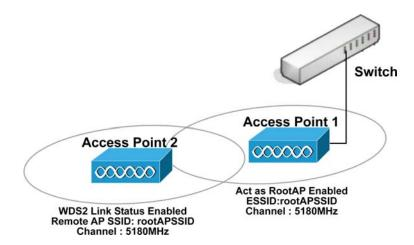
In this example, there are 2 access points: Access Point 1 and Access Point 2, with Access Point 1 as the root access point.
