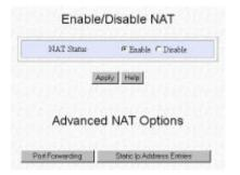
Figure 3.3.3-1 NAT Configuration Window for Static IP WAN Type
