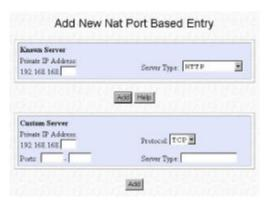
Figure 3.3.2-3 Defining New Virtual Server based on Port Forwarding
