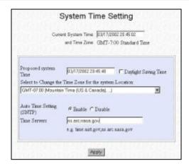
Figure 3.8.2-1 Synchronizing Router's Clock
