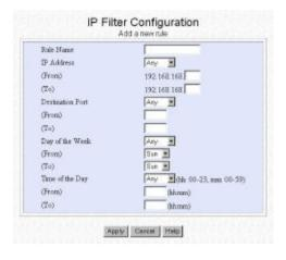
Figure 3.5.1-2 Defining Filtering Function
