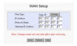
Figure 3.2.2-2 Static IP Configuration Page
