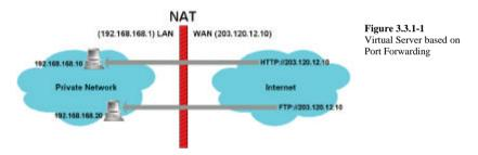
Figure 3.3.1-1 shows two Virtual Servers implemented, HTTP Virtual Server and FTP Virtual Server. To implement the Virtual Server, you need to know the TCP port that the intended application is using.
