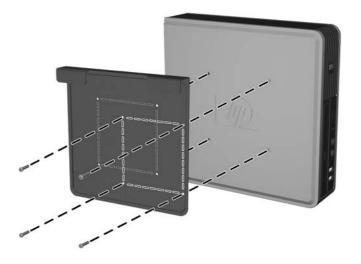
3. Slide the computer mounting bracket/USDT computer onto the stand (1) and reinstall the two screws on top of the bracket (2).
