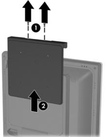
2. Remove the HP logo panel from the right side of the Thin Client to access the screw holes for the computer mounting bracket.
