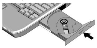
If your computer loses power, you can manually open the drive to remove a CD. Insert a straightened paper clip into the recessed hole on the front of the drive to open it.
