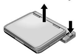
2. Lift the computer out of the port replicator.
