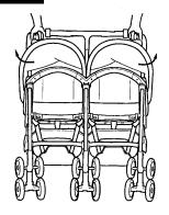
Grip the handle bar on each side and turn outward to open fully. (Holding from underneath will make the process easier.)
