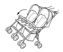
Lift up the handle bar and snap it away from you. It will open and automatically lock into position.
