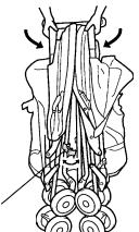
8. Lock the folding latch to hold the stroller together.
