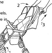
7. Fold together by bringing the sides of the handle together until the canopies face each other in the middle.
