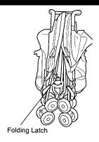
1. Release folding latch by pulling it forward.
