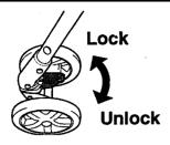
To lock swivels, lift all swivel lock levers up.
