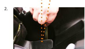
Slide wrench tool underneath lower end of plastic cover to pop open.
