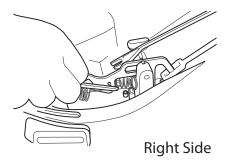
Using the slotted end of wrench tool provided, push hook and insert directly above current spring onto metal bracket as shown in figure 6b.
