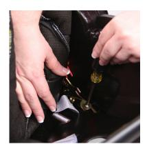
Place the assembled spring into the screw hole.
