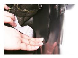
Reattach plastic cover and press down to snap in place as shown.
