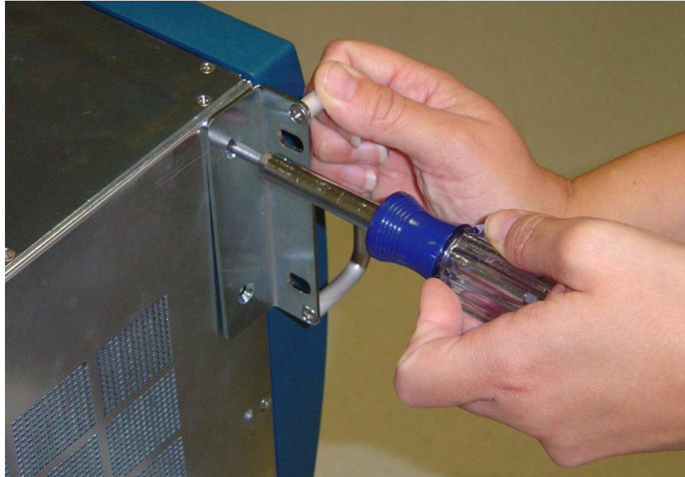
Figure 2-2: Unscrew Extra Rack Ears from the Chassis
