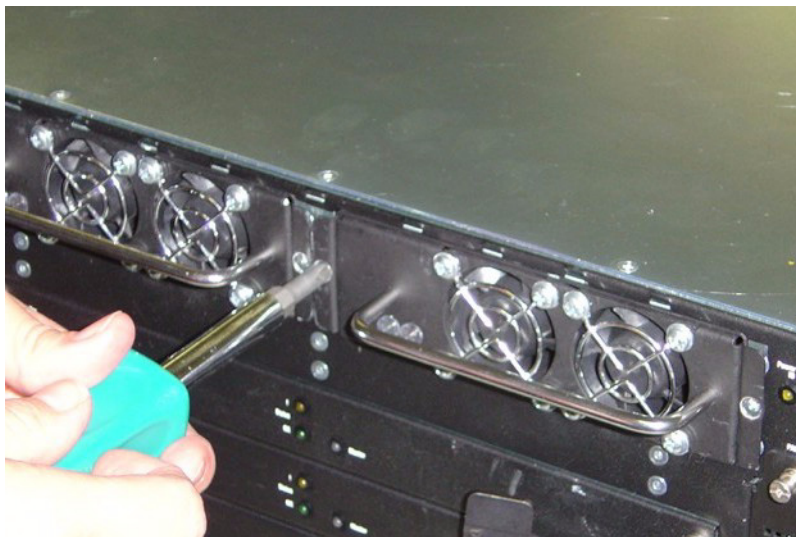
Figure 3-2: Loosening Captive Screws
