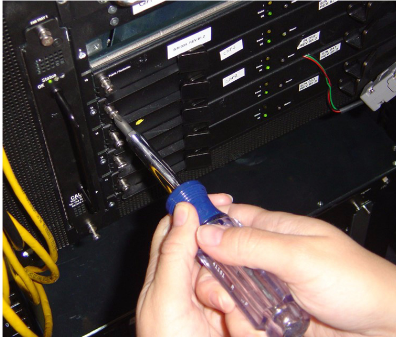
Figure 3-9: Loosen Captive Screws Before Removing
