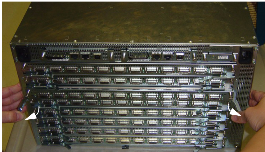
Figure 3-15: Releasing the LIM Module Levers
