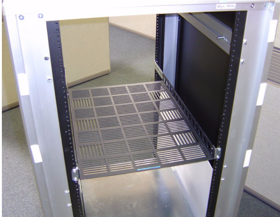
Figure 2-1: Install Appropriate Rack in Shelf
