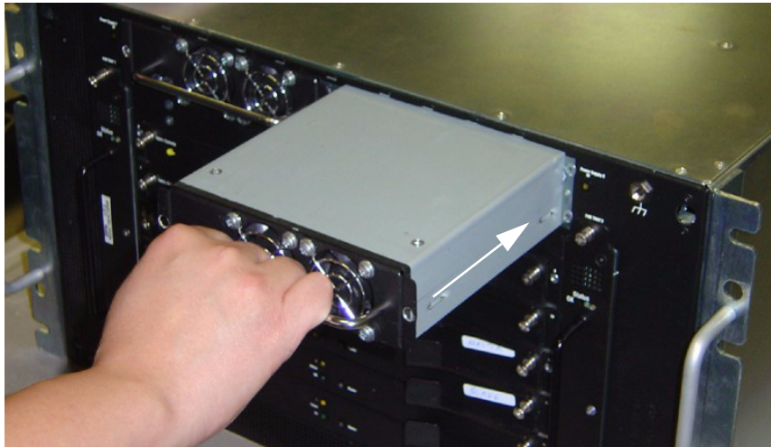
Figure 3-4: Inserting Power Supply Module
