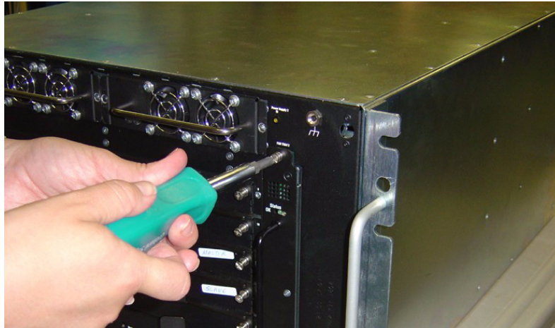
Figure 3-5: Loosening Captive Screws
