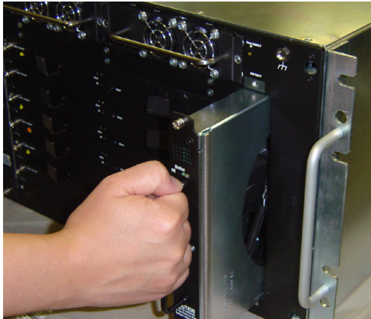
Figure 3-7: Pushing Fan Module into Slot
