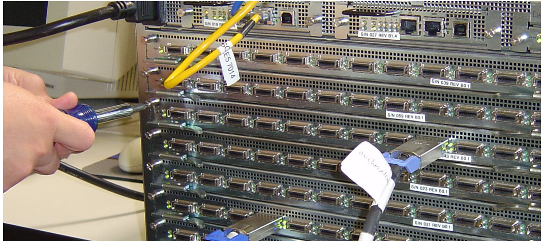
Figure 3-14: Loosen the Captive Screws
