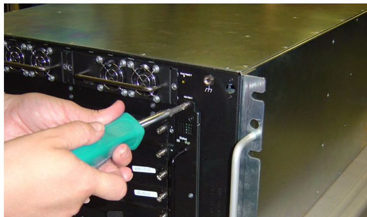
Figure 3-8: Tightening Captive Screws
