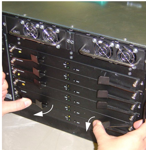
Figure 3-10: Opening Fabric Card Levers
