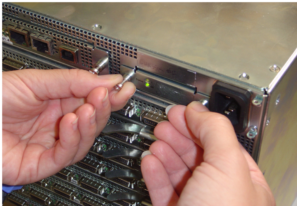
Figure 3-21: Remove the Chassis ID Module
