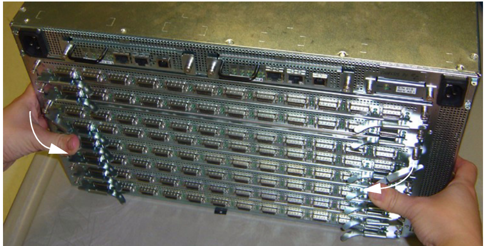
Figure 3-17: Closing the LIM Module Levers
