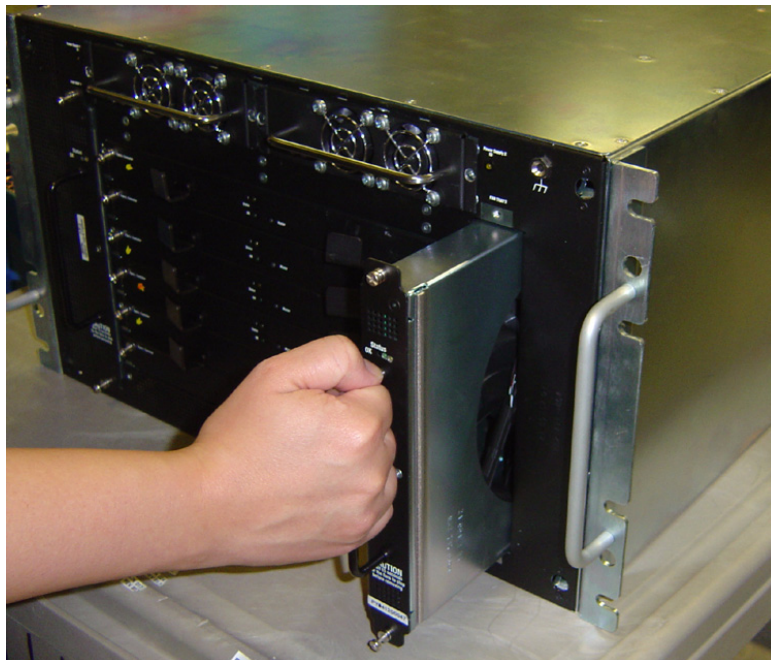
Figure 3-6: Partially Removing Fan Tray
