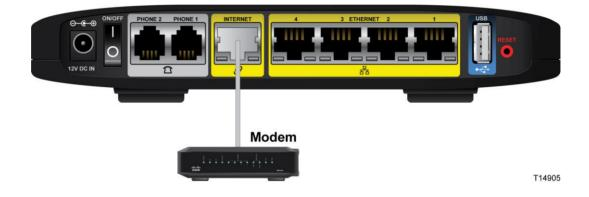
**3** Insert a standard RJ-45 Ethernet cable into an Ethernet port on the gateway and connect the other end to your PC.
