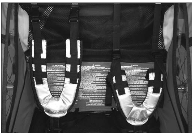
Comparison of different adjustments of the padded shoulder harness for children of different heights.
