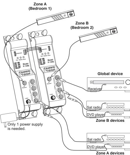
The diagram shown above, will create 2 IR zones that will allow for independent control of identical devices from the same manufacturer. The zone IR emitters will only respond to signals from the IR receiver that is in the same zone. The global IR emitters will respond to signals from any IR receiver in the system.
