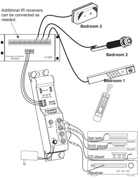
The diagram above illustrates how to create an IR system with IR receivers in several different rooms in the house. Systems like this may include several different styles of IR receivers depending on the specific application in each room.
