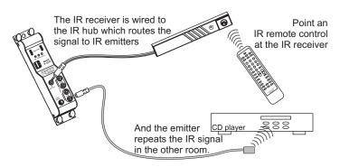
Be sure the emitter is attached directly over the component's IR receiver. To locate the IR receiver, shine a flashlight into the unit and look for the
