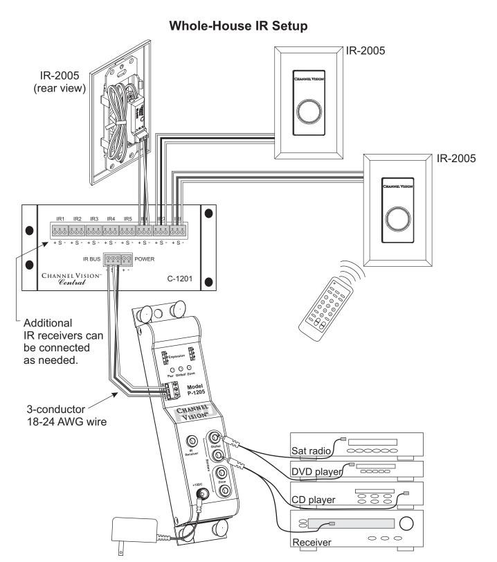
The diagram above illustrates how to create an IR system with IR receivers in several different rooms in the house. Systems like this may include several different styles of IR receivers depending on the specific application in each room.
