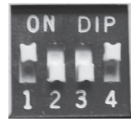
DIP SWITCHES SET TO '1001'
