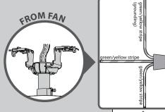
connector from the \*\pi hardware bag, connect the three grounding wires (green, green/yellow stripe, or bare copper) coming from the ceiling, downrod, and hanging bracket.
