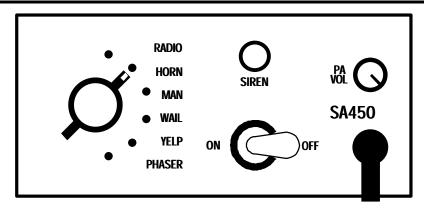
The **OFF/ON** Toggle Power Switch controls the siren power. The siren may be left on any time the vehicle is in operation. The power should be turned off when vehicle is not being used to conserve battery power.
